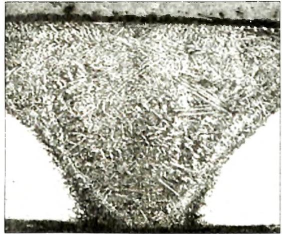
**Figure 3 : (Photomicrograph 2)** Fine Grained Dendritic Cast Structure of Metal in Fusion Zone, Magnification: x50, Etchant:: 10% Oxalic acid
