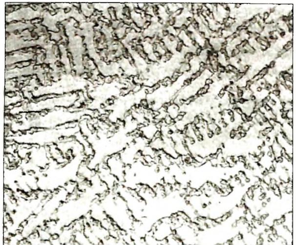
**Figure 6 : (Photomicrograph 5)** Laves Phase in the fusion zone of the weldment, Magnification: x1000, Etchant: 5% Chromic acid
