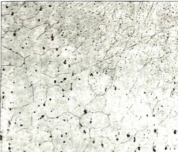
**Figure 6 : (Photomicrograph 5)** Fusion Zone Heat Affected Zone of welds made in solution treated specimen given post weld solution treatment, Magnification: x100, Etchant: 10% Oxalic acid
