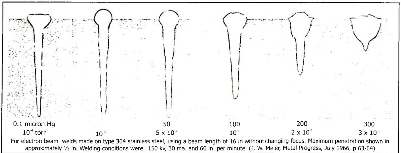
Fig. 1<sup>23</sup> Effect of welding-chamber pressure on penetration and weld shape
