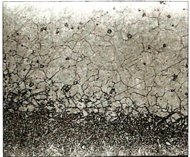
**Figure 5 : (Photomicrograph 4)** Segregation at Fusion Zone Heat Affected Zone, boundaries in solution treated specimen, Magnification: x100, Etchant: 5% Chromic acid
