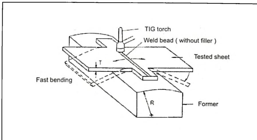
Figure 2 : Schematic representation of the set-up for Transvarestraint test unit
