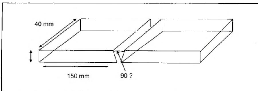
Figure 3 : Shows dimensions and edge preparation of specimen
