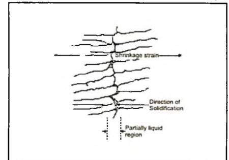
Figure 1 : Mechanism of Solidification Cracking
