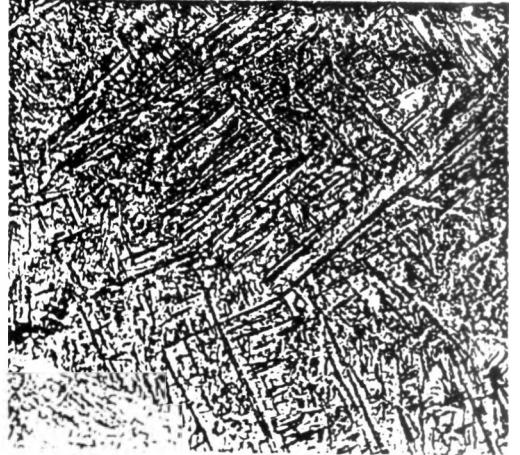
Fig. 4 : Microstructure of the fusion zone after post-weld heat treatment at 650°C (500X)
