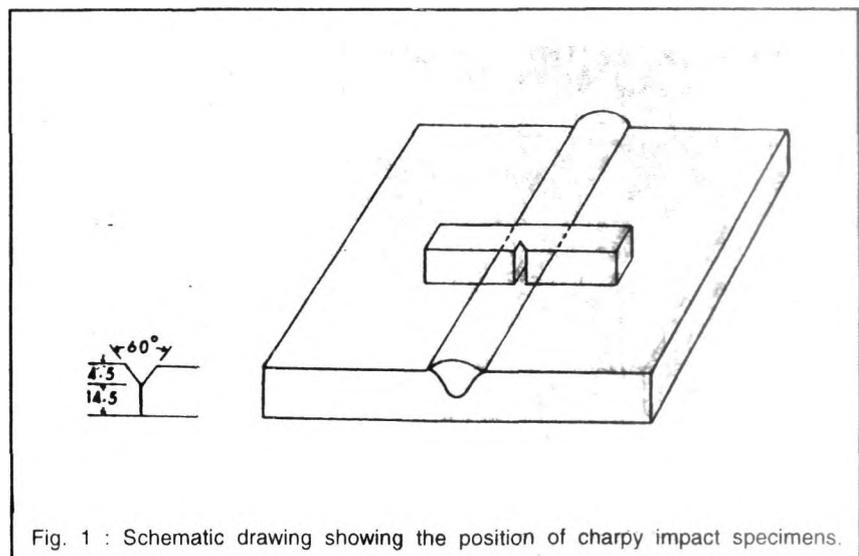
Fig. 1 : Schematic drawing showing the position of Charpy impact specimens.
