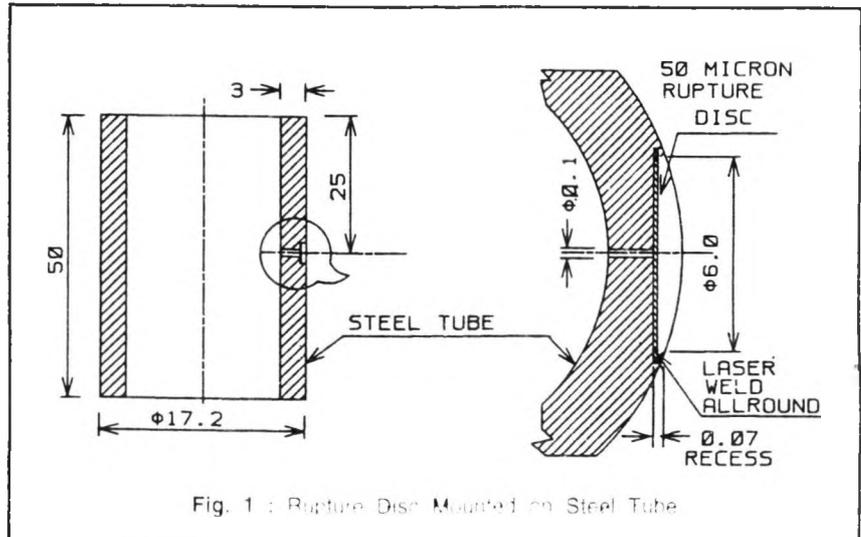
Fig. 1 : Rupture Disc Mounted on Steel Tube
