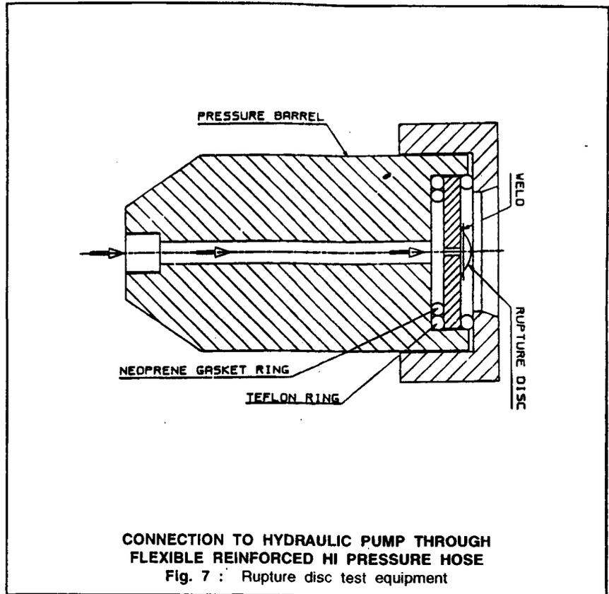
3. This development work has been progressing well. Since the rupture pressure is less than the requirement, the weld diameter needs to be reduced to about 6 or 7 mm to obtain the rupture
