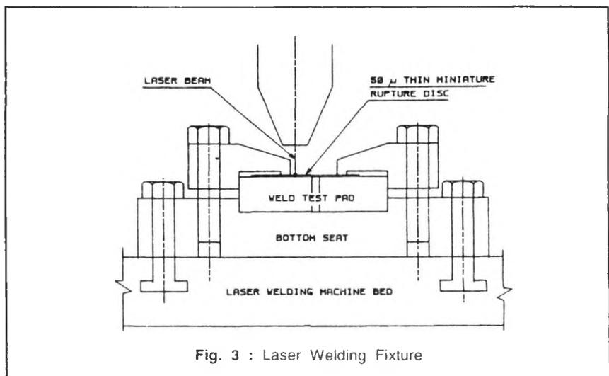
Fig. 3 : Laser Welding Fixture
