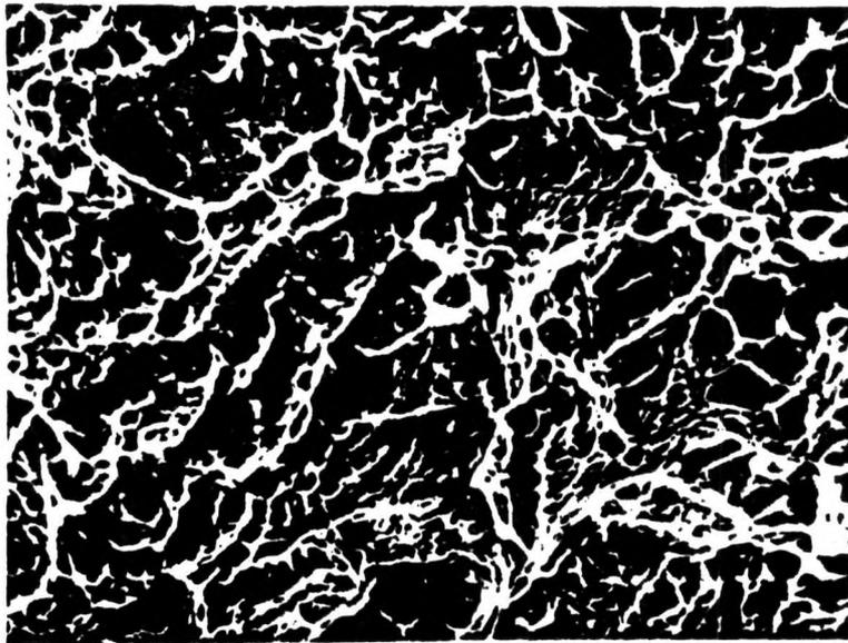
Fig. 7 : In-situ PWHT weld metal fractograph (SEM), 500X
