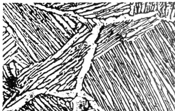
Fig. 4 : Weld metal PWHT, 1020°C, furnace cooled (optical) 500X
