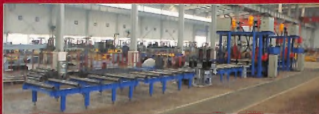
Horizontal assembly welding production line
