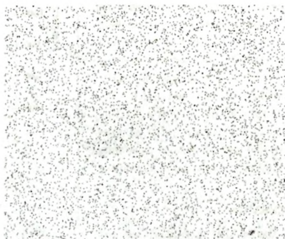
Fig. 15 : Ni element map shows enrichment of Ni along the lath boundaries
