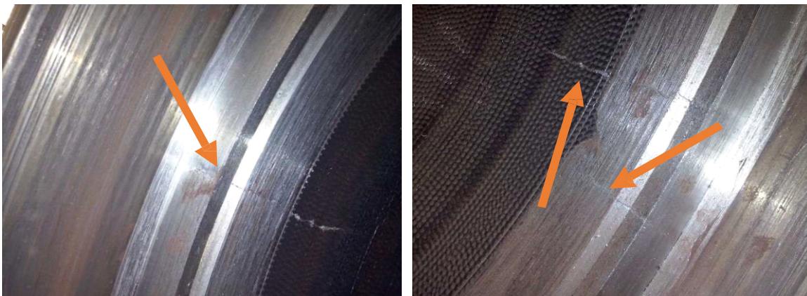
Fig. 8 : Delayed cracking in large diameter moulds
