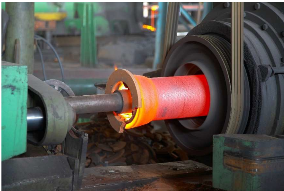
Fig. 1 : Centrifugal casting and extraction of ductile iron pipes
