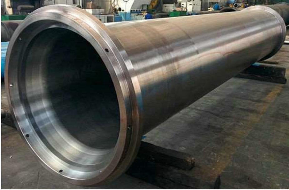
Fig. 3 : Typical mould employed in DIP manufacturing
