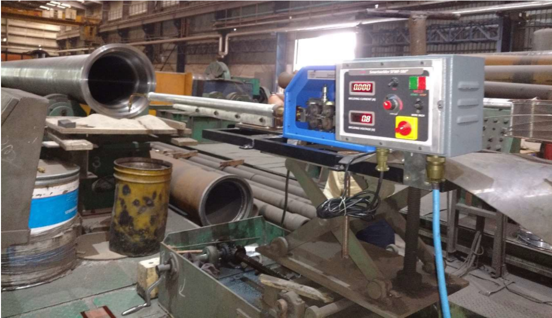
Fig. 7 : Sub arc welding set-up with a long gun
