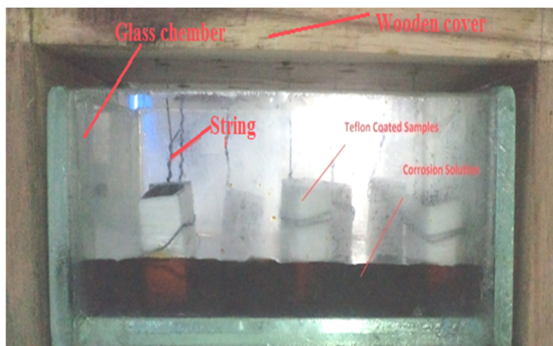
Fig. 5 : Corrosion test apparatus containing corrosive
