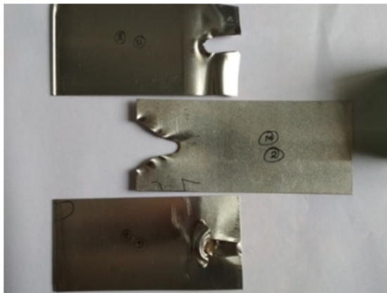
(a) Tested specimen at 12kA current with 40 cycles weld time and 2.5kg/cm 2 electrode pressure
