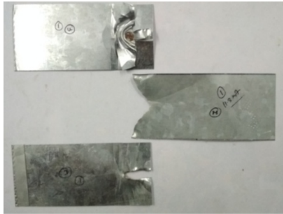
(a) Tested specimen at 14.85kA current and 2.5kg/cm 2 electrode pressure
