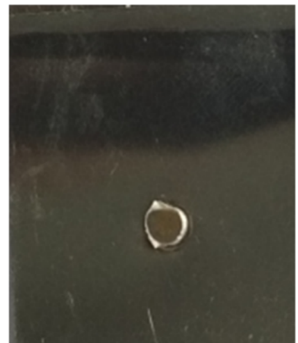
(c) Nugget size of triple stainless steel sheets joint
