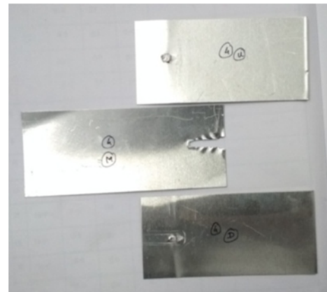
(b) Tested specimen at 12kA current and 1.5kg/cm 2 electrode pressure
