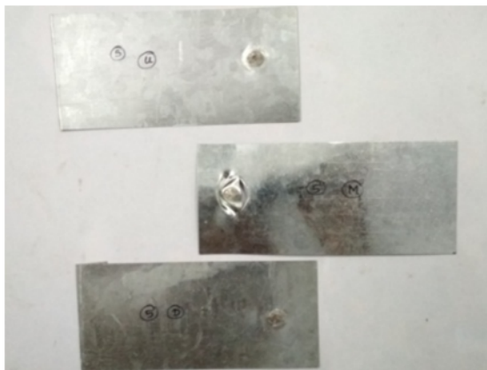
(c) Tested specimen at 13.5kA current with 40cycles weld time and 2.5kg/cm 2 electrode pressure
