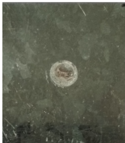
(b) Nugget size of triple galvanized iron sheets joint
