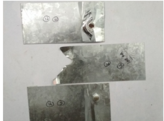
(b) Tested specimen at 14.25kA current and 1.5kg/cm 2 electrode pressure
