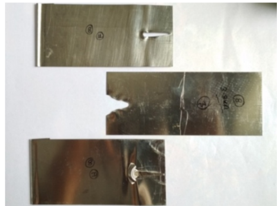
(b) Tested specimen at 12kA current with 20 cycles weld time and 1.5kg/cm 2 electrode pressure
