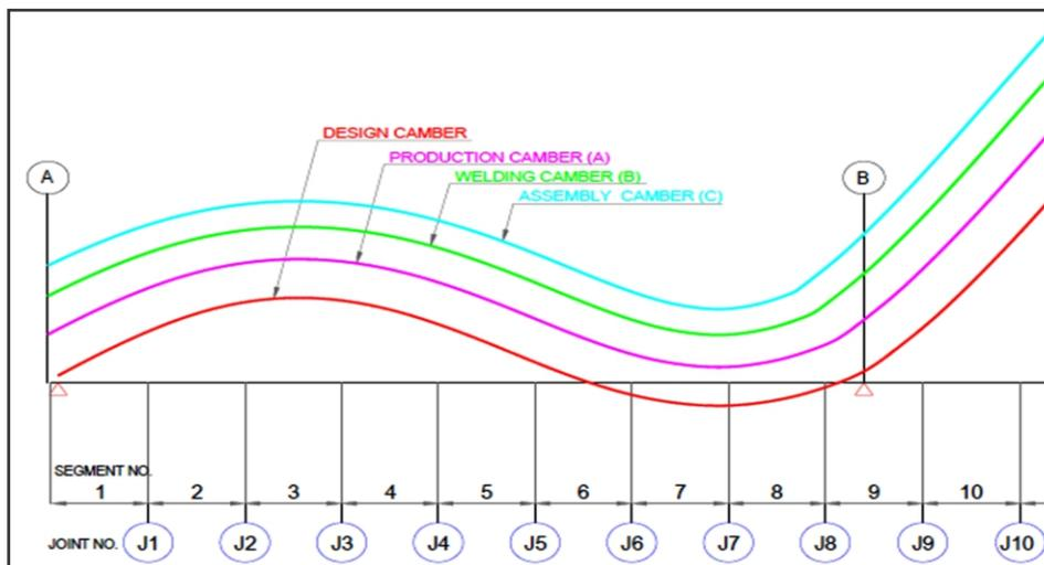
Fig. 6 : Diagram showing different cambers – (Between pier A & B)
