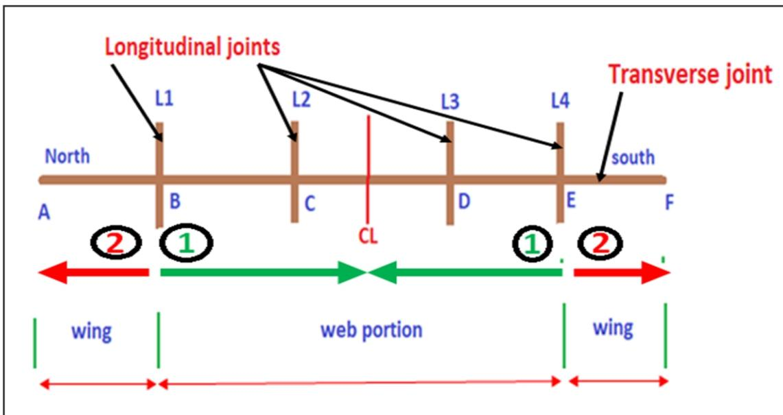
Fig. 23 : Modified welding sequences
