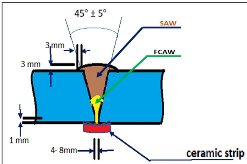
Fig. 5 : Schematic diagram of weld joint configurations
