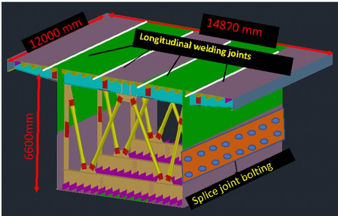
Fig. 2 : View of orthotropic steel deck (OSD) segment – After assembly
