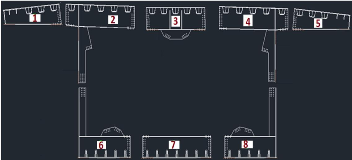
Fig. 1 : View of Orthotropic Steel Deck (OSD) blocks - Before assembly
