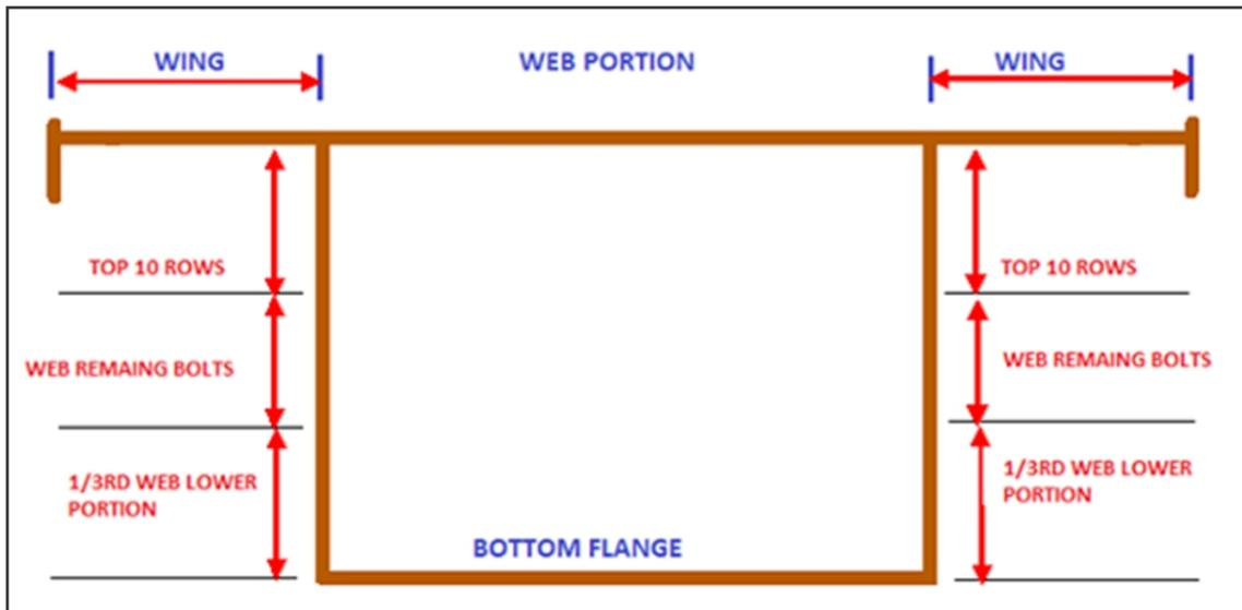
Fig. 20 : Bolting sequence details
