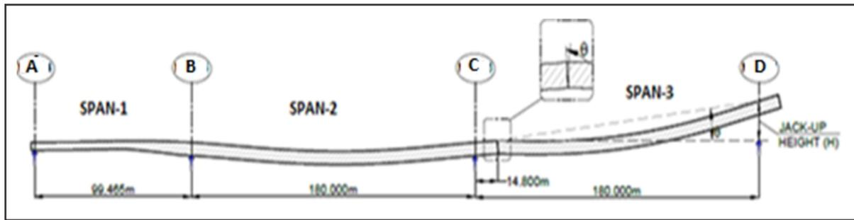
Fig. 19 : Span angular deformation (Indicative)
