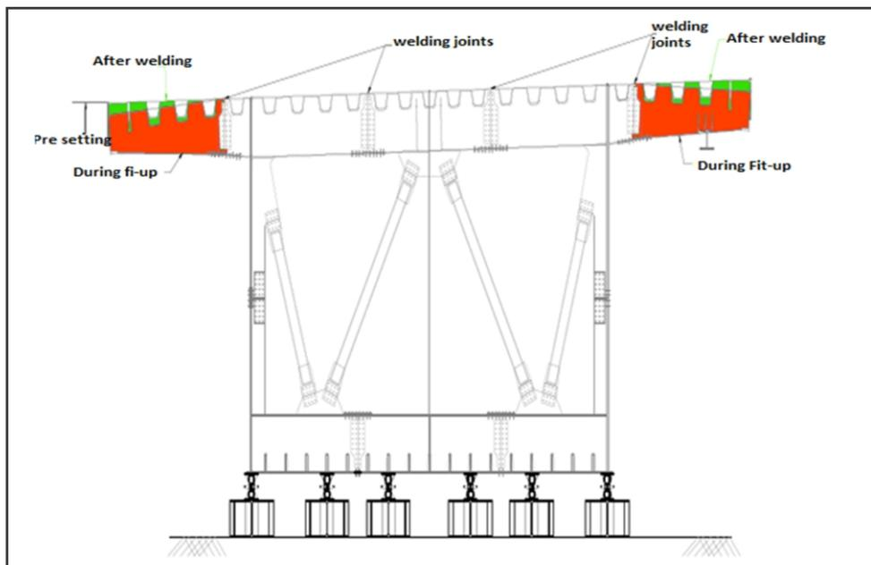
Fig. 16 : Presetting of Wings to avoid distortion
