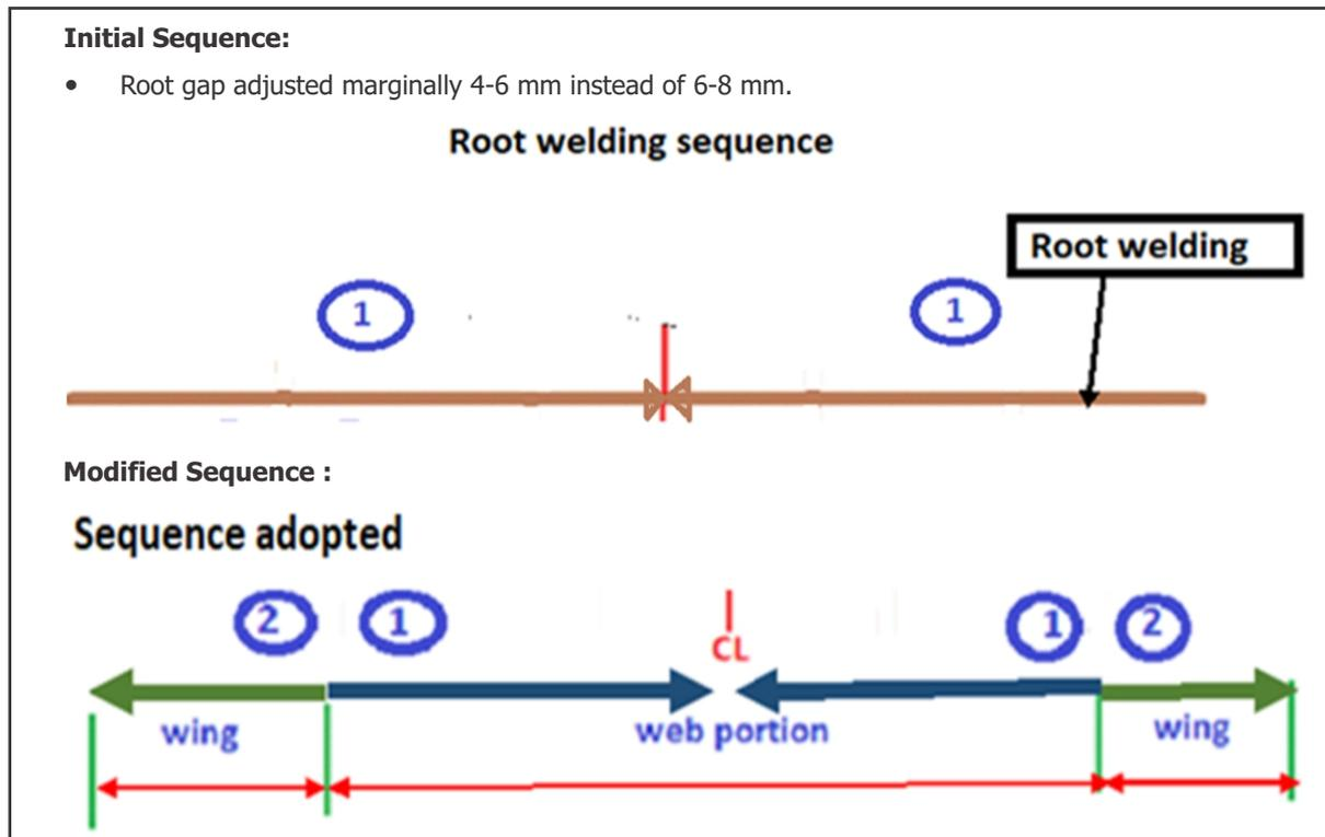
Fig. 17 : Initial & modified welding sequence
