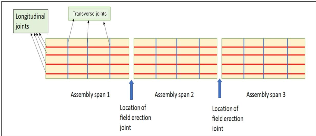
Fig. 3 : Key plan for weld directions
