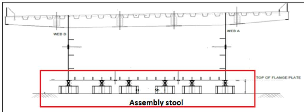
Fig. 9 : Provision of support stools for assembly– Section view
