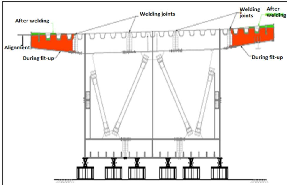
Fig. 15 : Upward distortion
