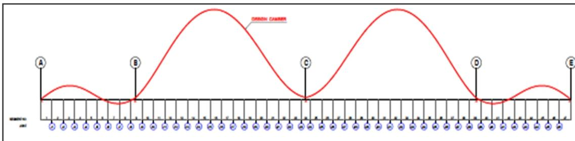
Fig. 7 : Design Camber across the spans – (Indicative)
