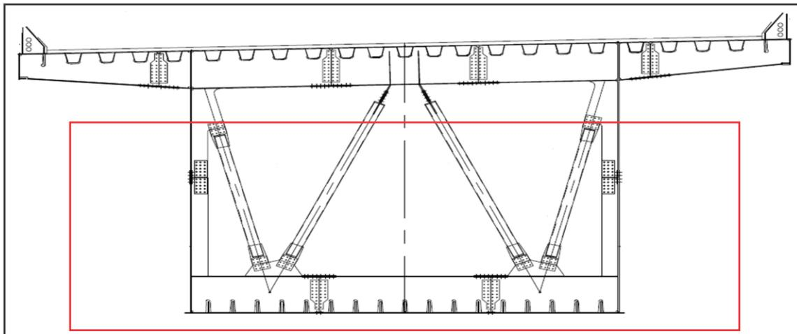
Fig. 10 : Bolt sequence before longitudinal direction welding
