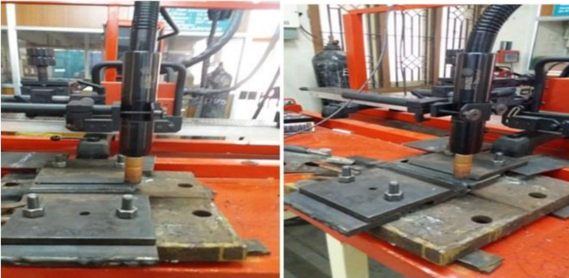
Fig. 3 : Rotating arc GMAW machine set up
