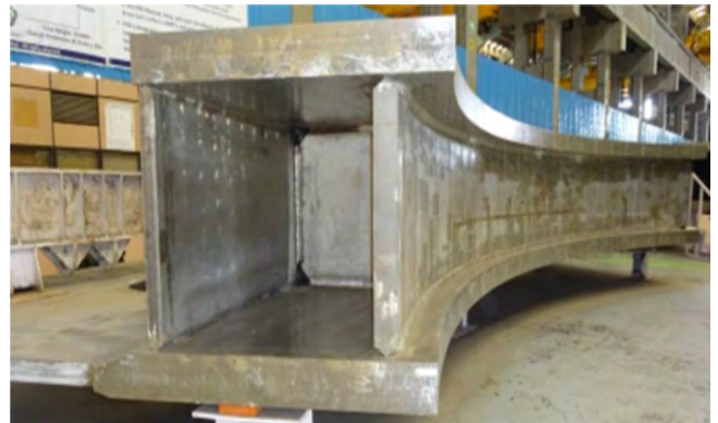
Fig. 8 : Base section Tier 2 Pedestal Ring in Factory
