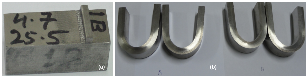
Fig. 9: (a) Shear tested, and (b) face-bend tested specimens of Ti/304L SS explosive cladded plates
