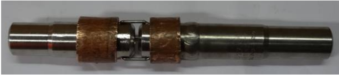
(b)Welding set-up with copper-sleeve as heat sink for fabrication of intermediate piece
