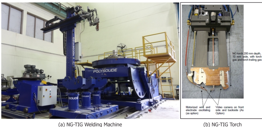
Fig. 1 : (a) Hot Wire Narrow-Gap TIG welding machine with column and boom arrangement and (b) NG-TIG Torch.
