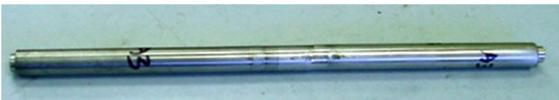
Fig.10 : Photograph of tensile test specimen of Ti/304L SS couple after TIG welding to Ti and 304L SS pipe
