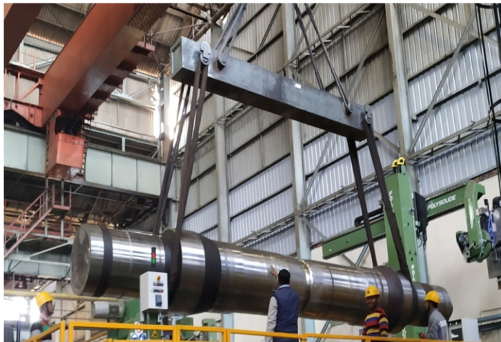
Fig. 4 : Photograph of Full Size AUSC Welded Rotor
