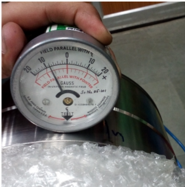
Fig. 3 : Checking magnetism prior to welding
