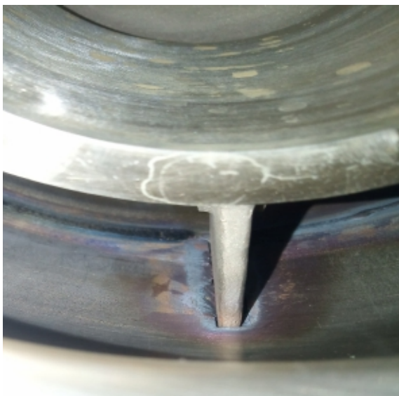
Fig. 11. : View of SS410 Rib to Casing joint
