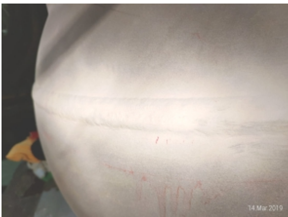
Fig. 7 : Indication of faint transverse crack in HAZ
