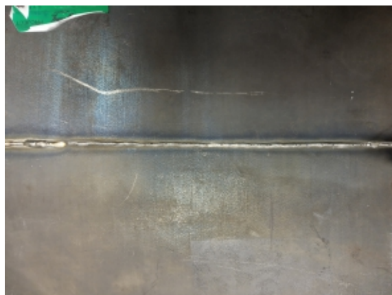
(b) Complete Joint Penetration
