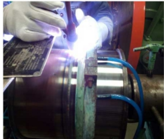
Fig. 2 : Photograph of dissimilar welding carried out
