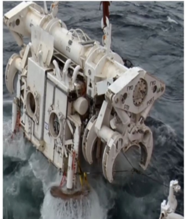
Fig.2 : Hyperbaric Welding Chamber [9]
