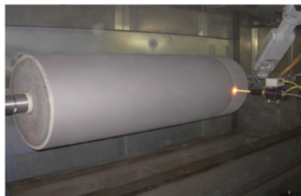
Fig.5 : One of the regular machine components coated with thermal spray powders
