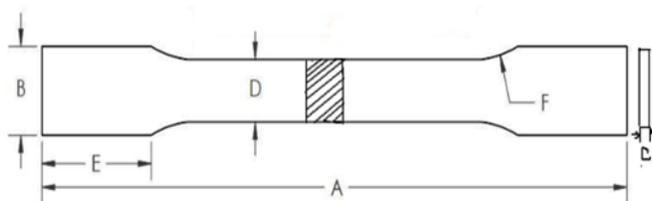
Where, A=100mm, B=10mm, C=3mm D=6.25mm, E=30mm, F=R6.25mm
