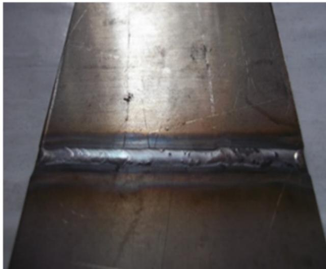
Fig. 2 : TIG welded duplex stainless steel sample
