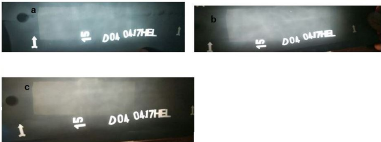
Fig. 4 : Welds processed with different pins (a) Triangle (b) Square and (c) pentagon
