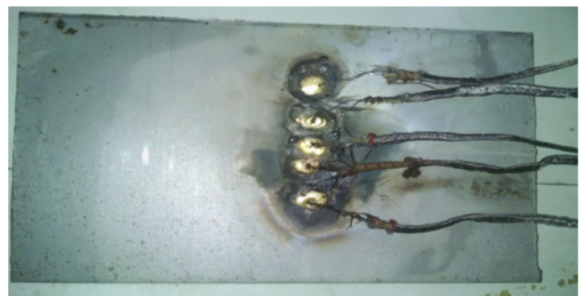
Fig. 5 : Thermocouples brazed onto the weld specimen
