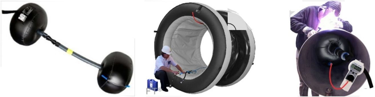
Fig. 7 : Above is Purge bladder- regular, custom made & with Monitor during welding in progress
