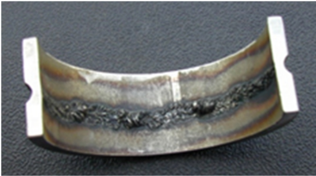
Fig. 2 : Bad root welding because of no purging
