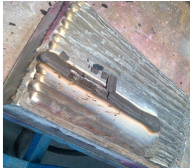
Fig. 8 : Dye-penetrant test after first layer of E 309 L H-FD. No indication of cracks or porosity
