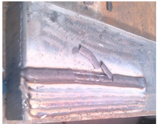
Fig. 9 : Good slag removal for E 347 H PW-FD
