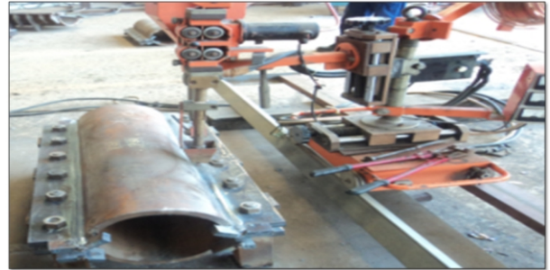
Fig. 7 : Riser Clamp joints by SAW
