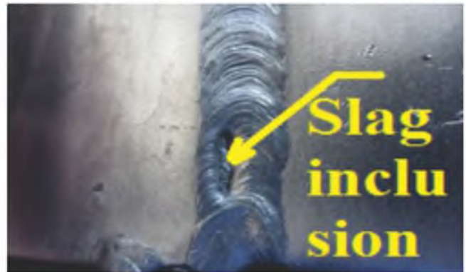
Fig.8 : Slag inclusion in a weld
