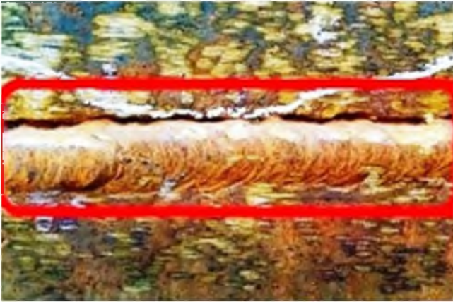
Fig.3 : Undercut in welding
