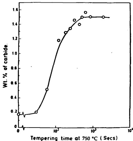
Fig. 15 variation of wt% of carbides vs tempering time at 750°C
