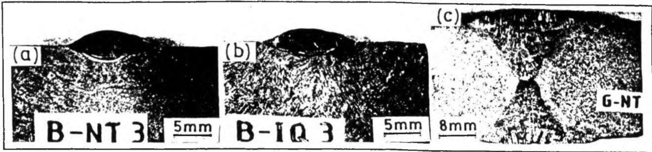
Figs. 10 Macrographs of post weld heat treated and aged (equivalent to 500°C/10 years) SMA weldments after potentiostatic etching (a) N&T-0.66 kJ/mm, (b) IQ-0.66 kJ/mm, (c) N&T-0.83 kJ/mm (multipass)
