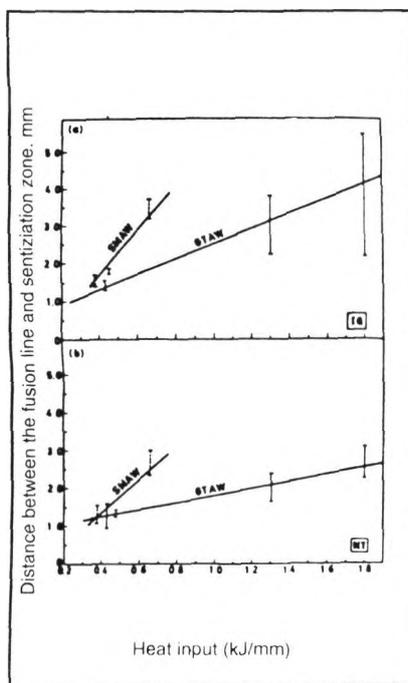
**Fig. 4** Variation of the distance between fusion line and sensitization zone as a function of heat input (a) IQ, (b) N&T
