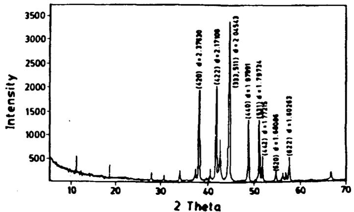
Fig. 16 Diffractograph of the precipitate obtained in electrochemical extraction
