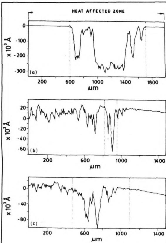
Fig. 7 Surface profile over the etched weldments prepared from ice-quenched 9%Cr-1%Mo steel (a) 0.48 kJ/mm, (b) 1.3 kJ/mm, (c) 1.8 KJ/mm
