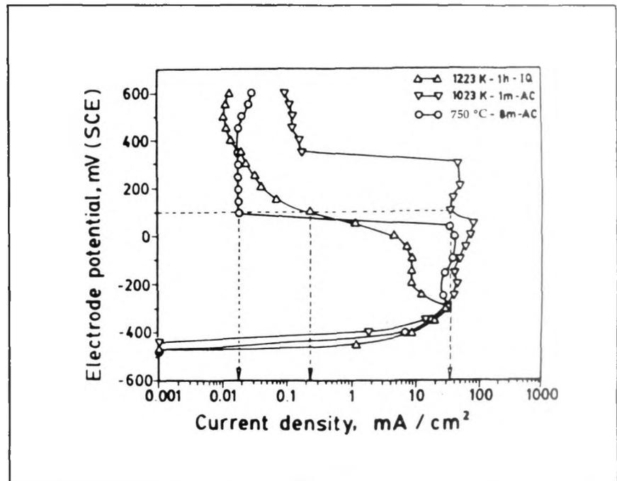
Fig. 1. Anodic polarisation curves for 9%Cr-1%Mo steel in 16 wt.% H<sub>2</sub>SO<sub>4</sub> solution
