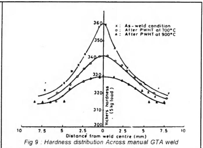
Fig 9 : Hardness distribution Across manual GTA weld
