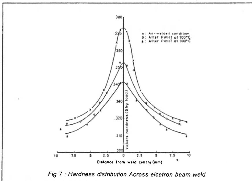
Fig 7 : Hardness distribution Across electron beam weld
