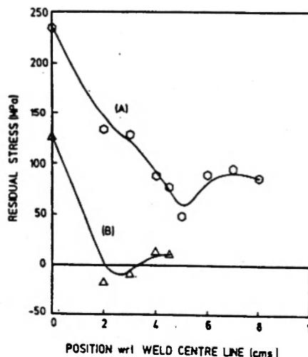
Fig 10 : XRD Residual stress across root pass in 12mm Thick Weld Joint
