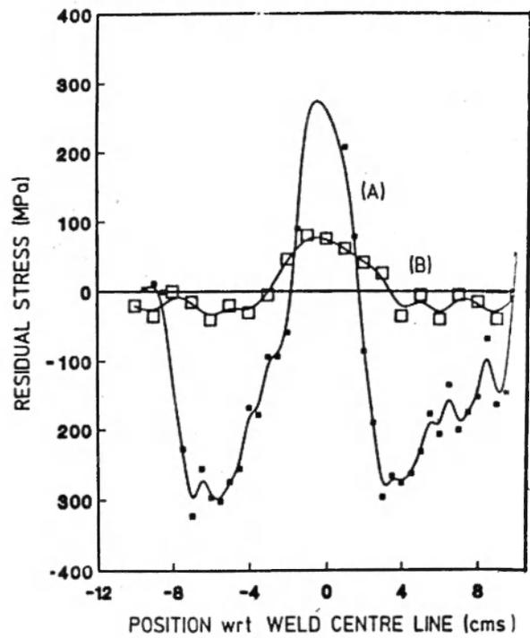
Fig 12 : Effect of annealing on the thickness Averaged Residual Stress measured by ultrasonic technique in 8mm thick plate. (a) As welded (b) 873K Anneal
