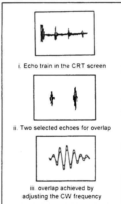
Fig 4 : Sequence of overlap of any two echoes in ultrasonic velocity measurement
