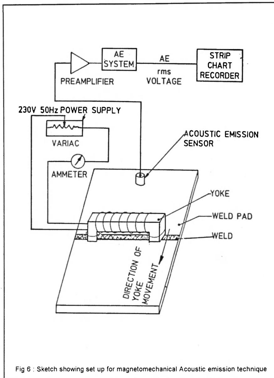
Fig 6 : Sketch showing set up for magnetomechanical Acoustic emission technique
