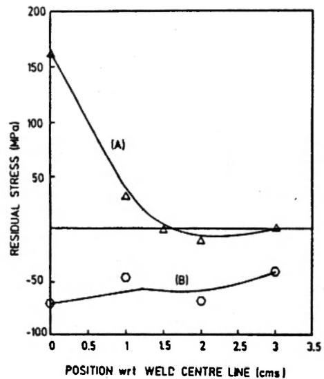
Fig 8 : XRD Residual stress across root pass in 8mm, Thick Weld Joint
