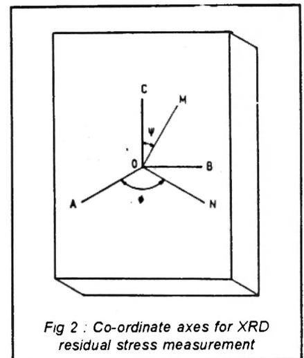
Fig 2 : Co-ordinate axes for XRD residual stress measurement
