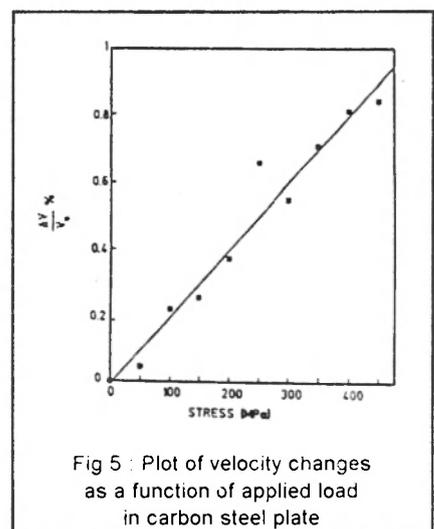
Fig 5 : Plot of velocity changes as a function of applied load in carbon steel plate
