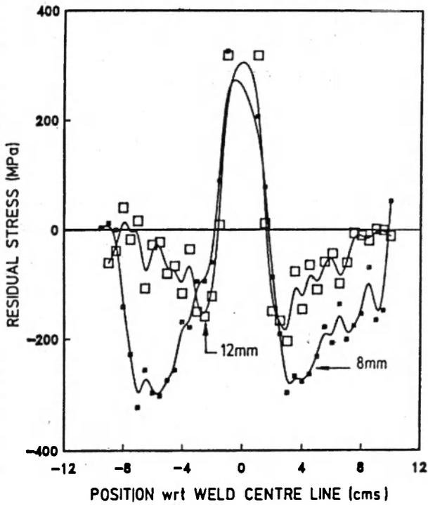
Fig 11 : Thickness Average Residual Stress variation measured by ultrasonic technique in as welded 8mm and 12mm thick mild steel plates
