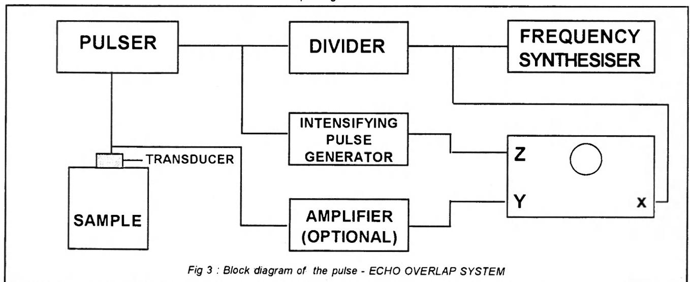
Fig 3 : Block diagram of the pulse - ECHO OVERLAP SYSTEM
