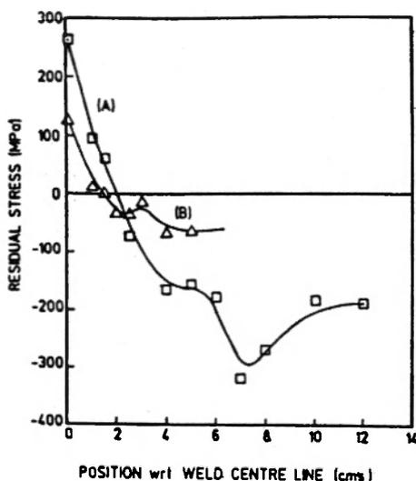
Fig 9 : XRD Residual stress on top surface of 12mm Thick Weld Joint
