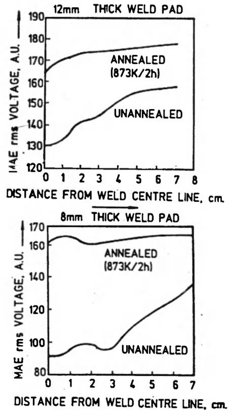
Fig 14 : Variation in MAE with distance from weld centre line
