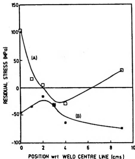
Fig 7 : XRD Residual stress on top surface of 8mm Thick Weld Joint
