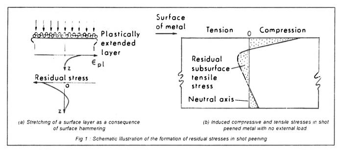
vary. Depth is important and the shot-peening parameters are chosen to suit the problem. For instance should the environment not be excessively corrosive or suffer erosion and be reasonably smooth or defect free then a shallow compressive layer is adequate. However, excessive corrosion, erosion or surface defects require maximum depths of cold work otherwise limited benefit will be noted.
