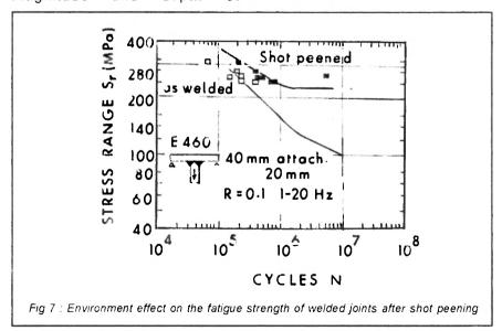
In applications where the critical stress levels are known and thermal stress relief is adequate even though 15-20% of the HAZ stress can still be present after treatment, then CSP can often be preferential on economic grounds only. In other words the technique can be used as a stress relieving operation where the residual compressive stress induced is a bonus but not essential. Local CSP has shown considerably cheaper on many structures than thermal stress relief
