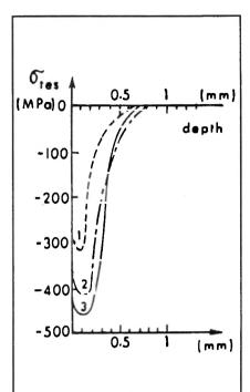
Fig 5 : Distribution of shot-peening stress with depth for different shot peening operations
