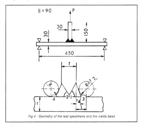
or the weld micro structure [6]. Because of the insignificant effect of the yield strength of steel on fatigue crack growth, the only way of taking full advantage of steels of high characteristics is to increase the part played by crack initiation in the total life of the welded assembly. For this purpose CSP can be used with the purpose of modifying the range of residual stresses introduced by welding. There is little information on results in
