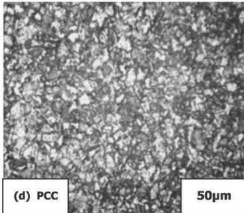
Fig. 6 : Optical micrographs of Stir zone
