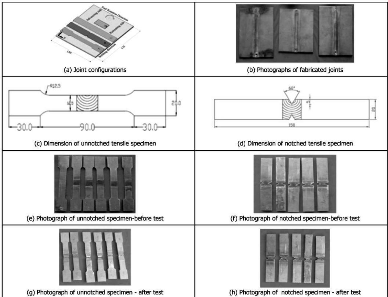
**Fig.2 : Fabrication of joints and tensile specimen**
