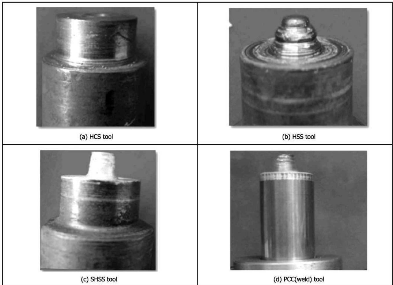
**Fig. 3 : Appearance of the tools after FSW of copper**
