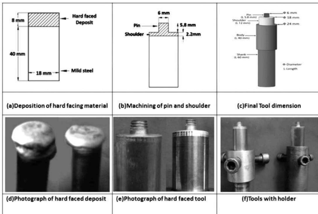
Fig. 1 : Schematic representation of hardfaced tool fabrication
