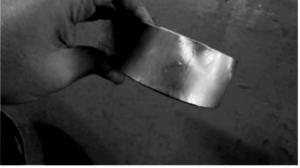
Bend test sample prepared from web portion of the Rail section. Test conducted as per ASME Sec-XI Clause QW 160 guideline but no crake observed in weld zone, hence accepted.
