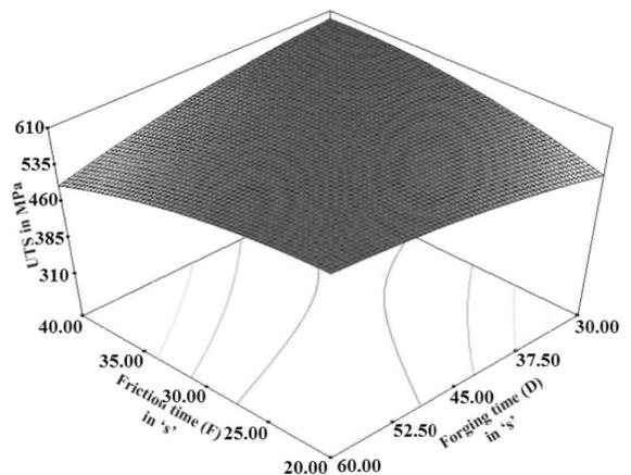
c. Response plot showing the effect of F and D on tensile strength at R = 2112.23 RPM
