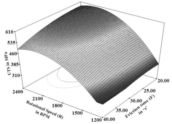
a. Response plot showing the effect of R and F on tensile strength at D = 55.1 s
