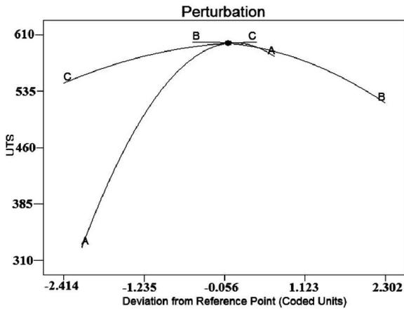
Fig. 4 : Perturbation plot showing the effect of all factors on the tensile strength
