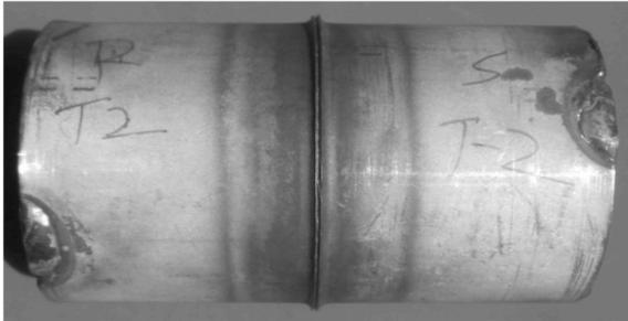
a. Photograph of friction welded tube joint
