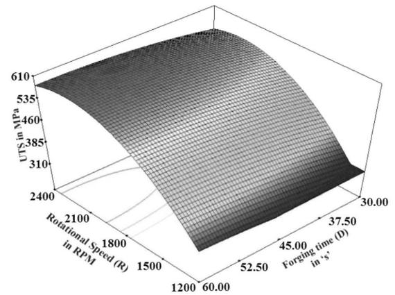
b. Response plot showing the effect of R and D on tensile strength at F = 23.73 s
