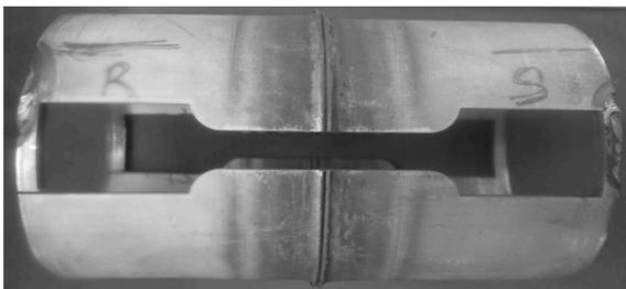
b. Scheme of specimen extraction
