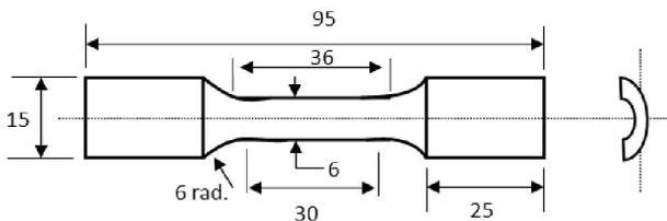
c. Schematic representation of tensile specimen
