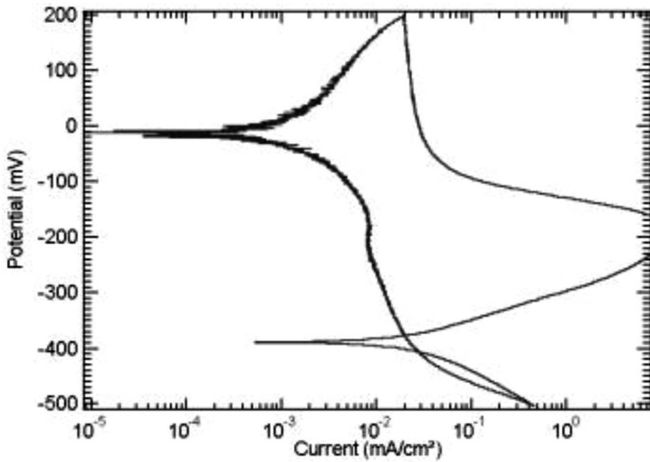
Fig. 7 : Double-loop EPR curve of the specimen cladded at 2.49 KJ mm<sup>-1</sup> Conditions
