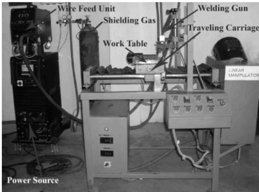
**Fig. 1 : Weld cladding experimental setup**
