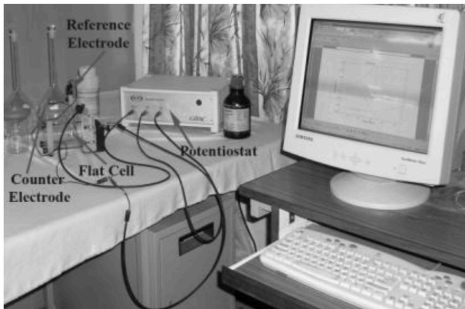
**Fig. 3 : Experimental setup used for corrosion study**
