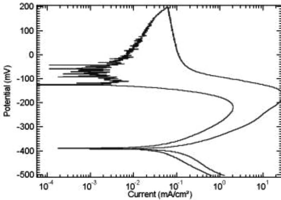
Fig. 4 : Double-loop EPR curve of the specimen cladded at 0.82 KJ mm<sup>-1</sup> conditions
