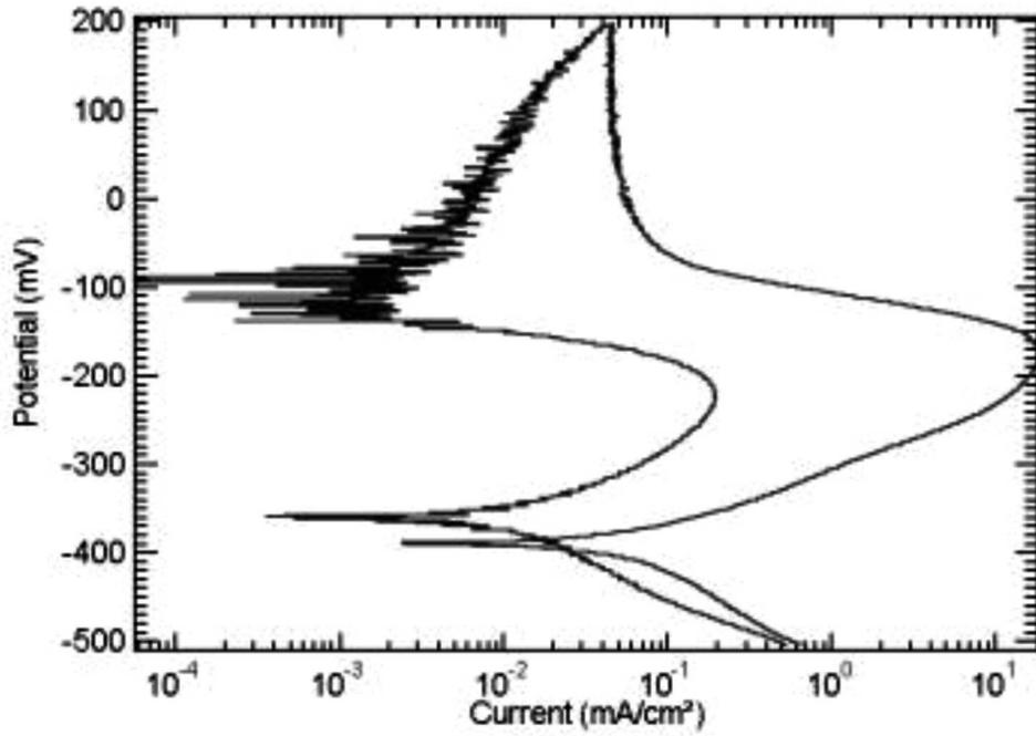
Fig. 6 : Double-loop EPR curve of the specimen cladded at 1.40 KJ mm<sup>-1</sup> Conditions
