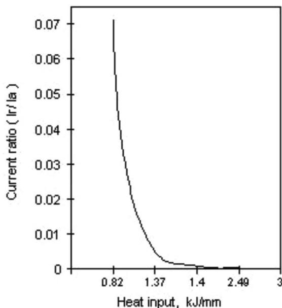
**Fig. 8 : Effect of heat input on Intergranular corrosion resistance**
