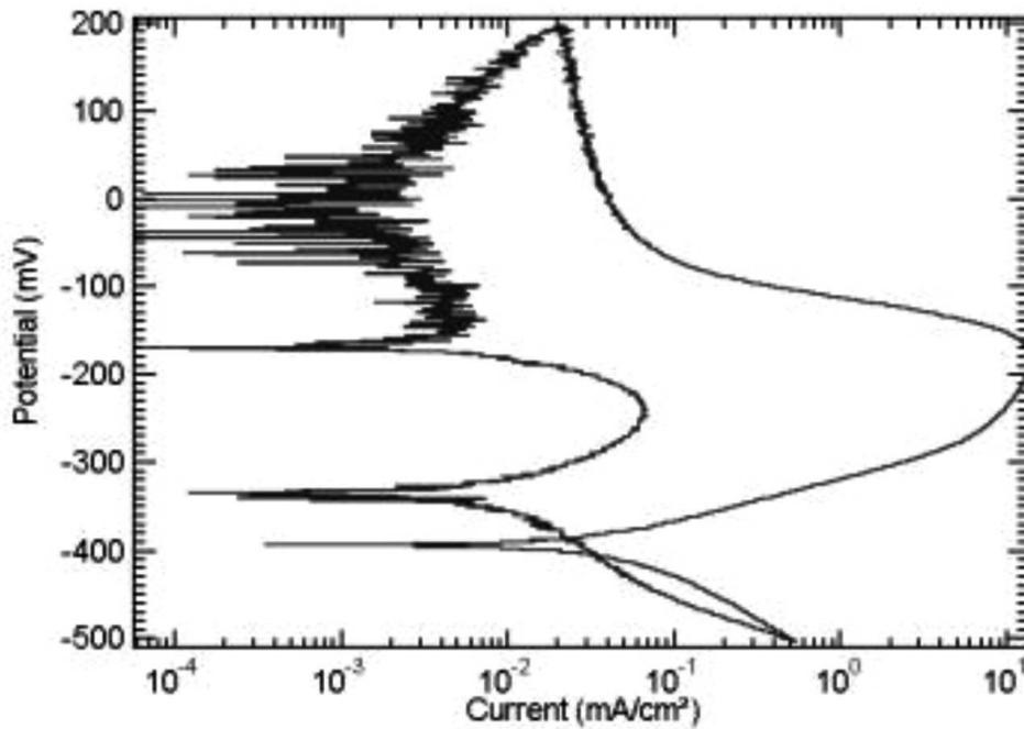
Fig. 5 : Double-loop EPR curve of the specimen cladded at 1.34 KJ mm<sup>-1</sup> conditions
