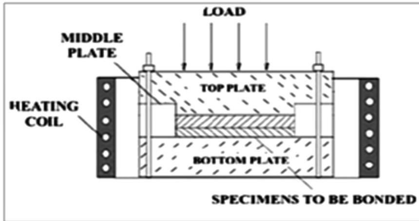
**Fig 1: Configuration of the diffusion bonding die set up**
