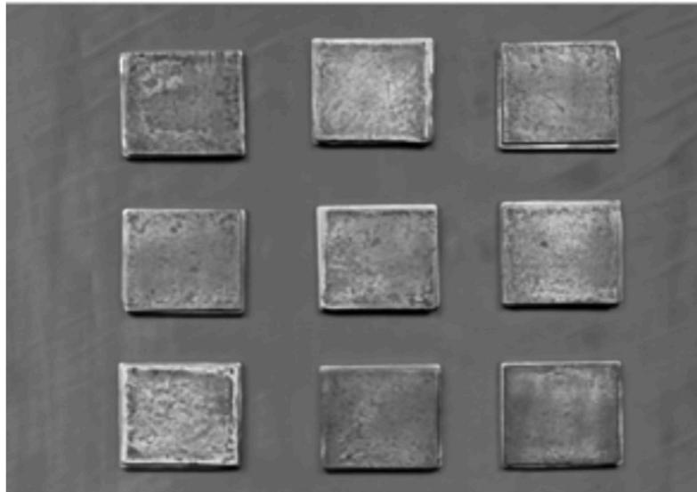
**Fig. 2 : Photograph of few of the fabricated diffusion bonds**
