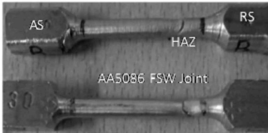
**Fig. 6 : Fractured tensile specimens of FSW joints**
