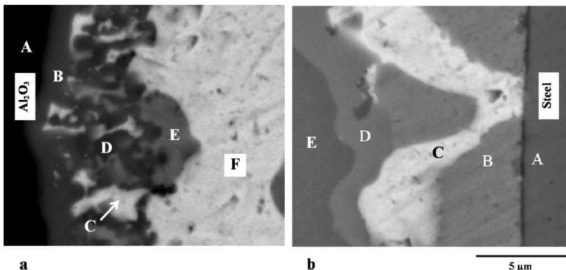
Fig. 2: SEM BSE images of 15 min brazed joint (a) alumina interface and (b) En24 interface.
