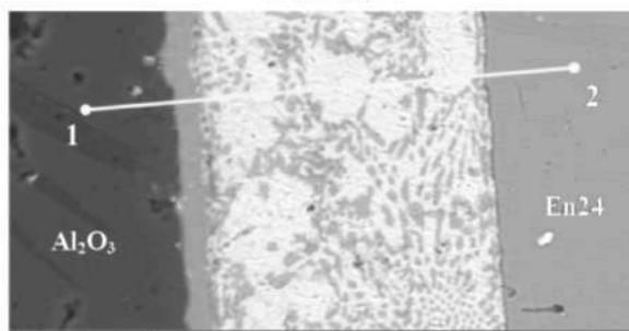
Fig. 8: EPMA X-ray intensity line map of 45 min brazed joint.
