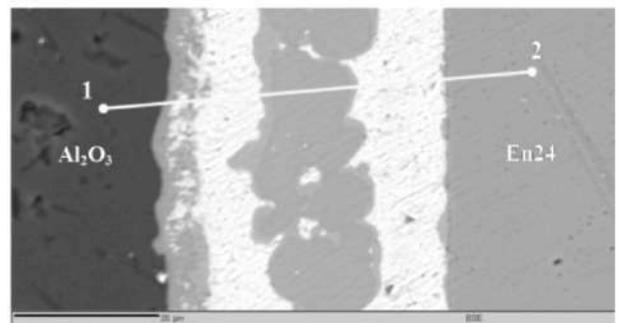
**Fig. 6: EPMA X-ray intensity line map of 15 min brazed joint.**
