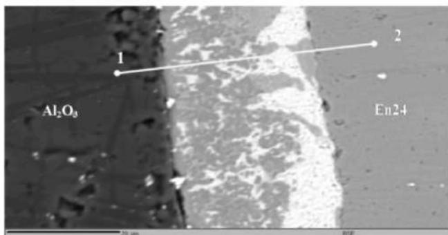
Fig. 7: EPMA X-ray intensity line map of 30 min brazed joint.
