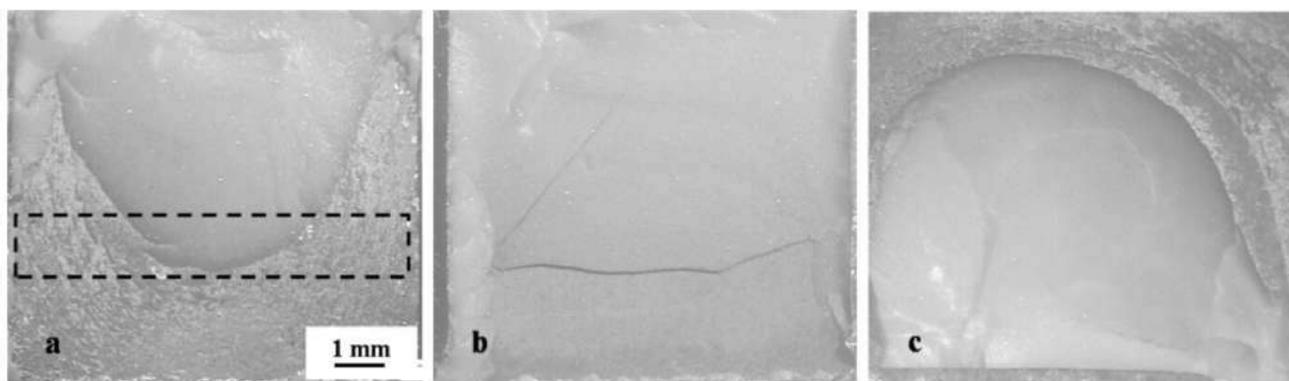
**Fig. 14: Optical images of fractured surfaces of joints brazed at 850°C for (a) 15 min (b) 30 min and (c) 45 min.**
