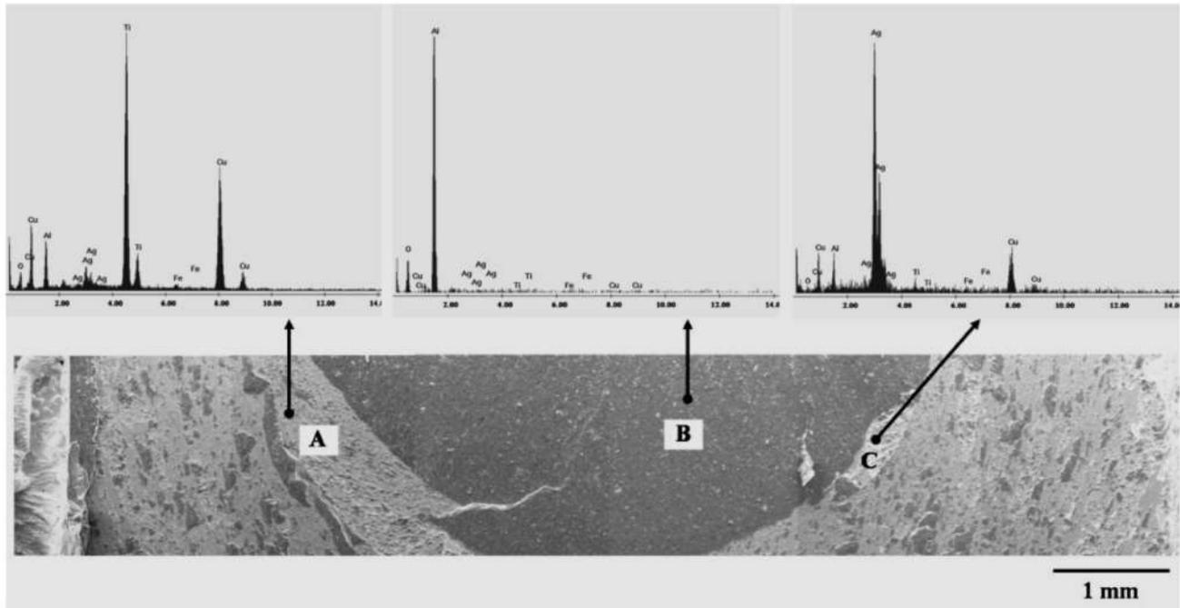
**Fig. 15: SEM image of fractured surface of joint brazed for 15 min. EDS analysis of three major regions: A –  $(Al,Ti)_2O_3$ ,  $CuAlO_2$ ; B –  $Al_2O_3$ ; C – Ag solid solution.**
