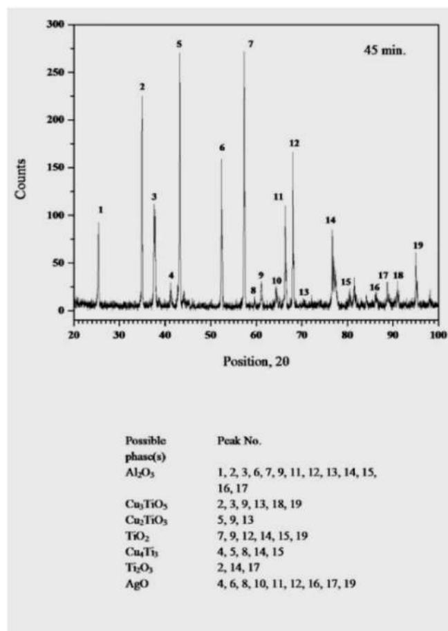
**Fig. 13: XRD Analysis of 45 min brazed joint.**
