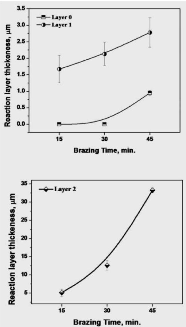
**Fig. 5: Variation of reaction layers thickness with respect to brazing time.**
