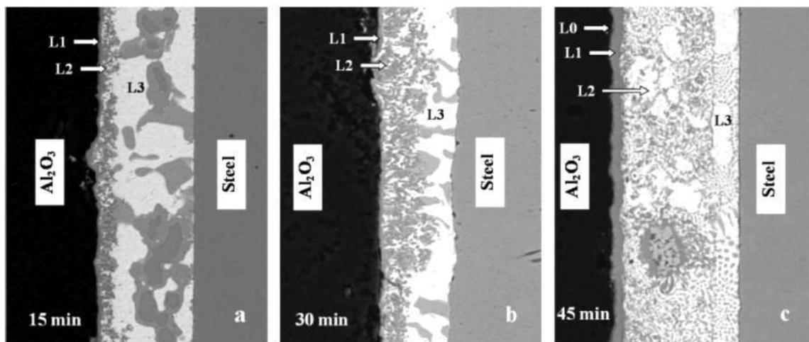
**50 µm** Fig. 1: SEM BSE images of alumina-steel joints vacuum brazed at 850°C for (a) 15 min (b) 30 min and (c) 45 min.
