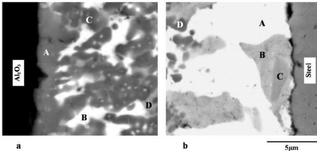
**Fig. 3: SEM BSE images of 30 min brazed joint (a) alumina interface and (b) En24 interface.**
