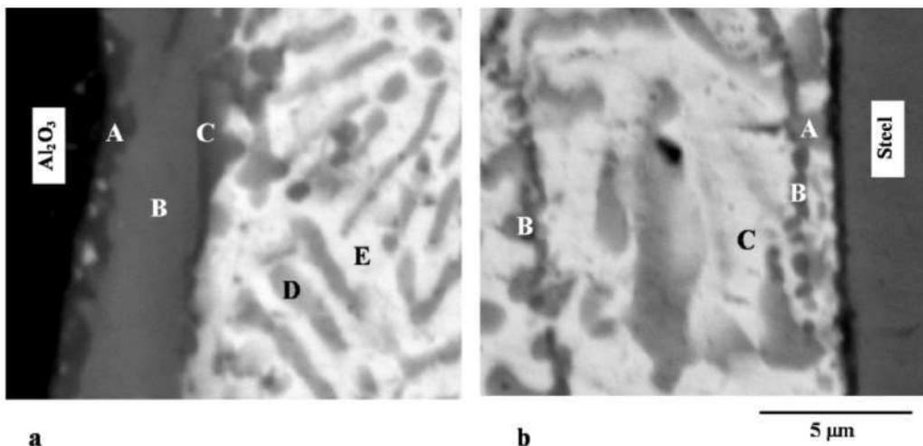
**Fig. 4: SEM BSE images of 45 min brazed joint (a) alumina interface and (b) En24 interface**
