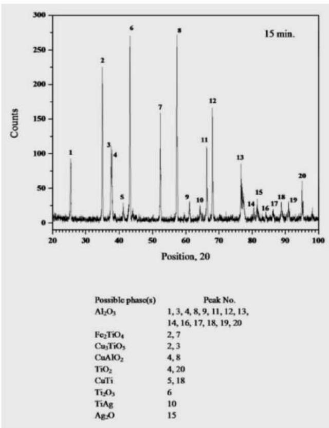
Fig. 11: XRD Analysis of 15 min brazed joint.
