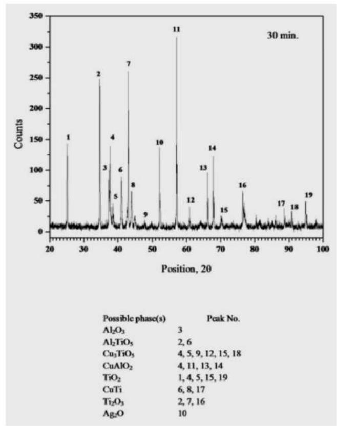
Fig. 12: XRD Analysis of 30 min brazed joint.
