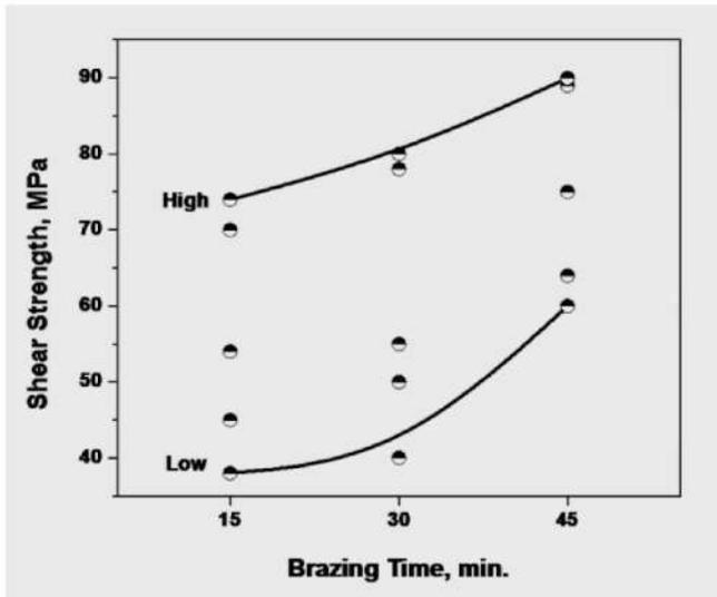
Fig. 10: Variation of lap shear strength with respect to brazing time.
