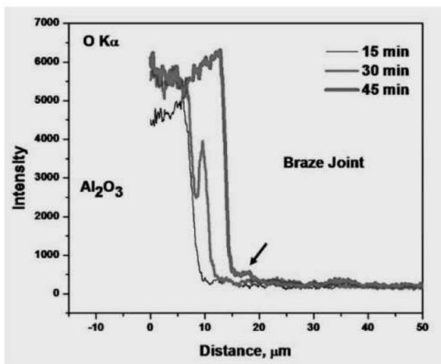
Fig. 9: Variation of O with respect to brazing time at  $Al_2O_3$  interface.
