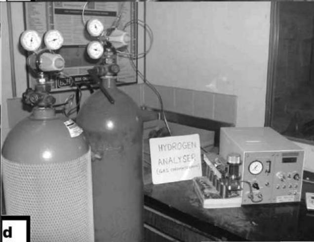
Fig. 7 Oerliken-Yanaco GC setup for HD measurement (Photo Courtesy: [54]) a)Flow Diagram of GC apparatus b) Electric Furnaces to heat chamber c) Chambers Connected to GC analyzer d) Carrier gas connected to GC analyzer
