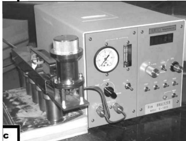
Fig. 7 Oerliken-Yanaco GC setup for HD measurement (Photo Courtesy: [54]) a)Flow Diagram of GC apparatus b) Electric Furnaces to heat chamber c) Chambers Connected to GC analyzer d) Carrier gas connected to GC analyzer
