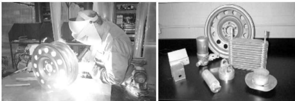
Fig.6 : Some automotive components in Aluminium that have been repaired by welding
