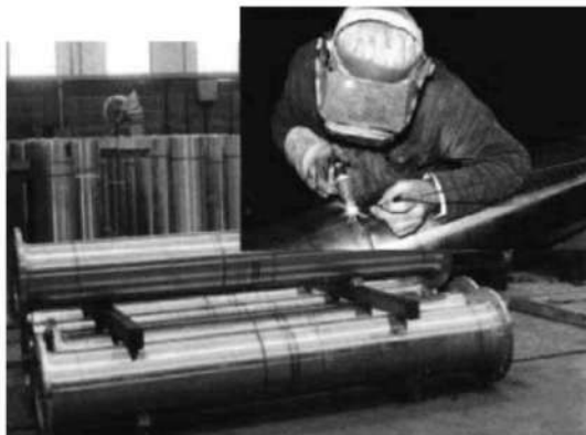
Fig. 8 : Aluminium Bronze Pipe welding
