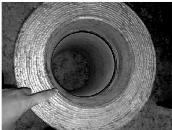
Fig. 7 : Some of the overlay components with Nickel Alloys & Welding of a Gas Turbine part made of Alloy 617
