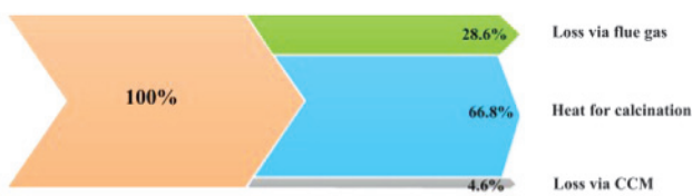
Energy efficiency of TBFC is 66.8%, almost doubly higher than 33.9% of traditional RF
