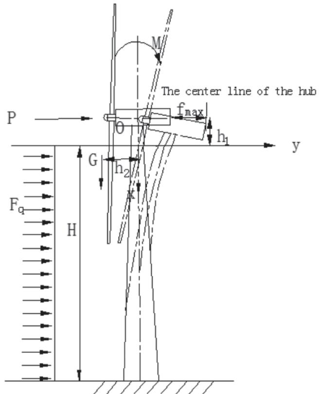
Fig.6: The mechanical model of wind turbine tower
