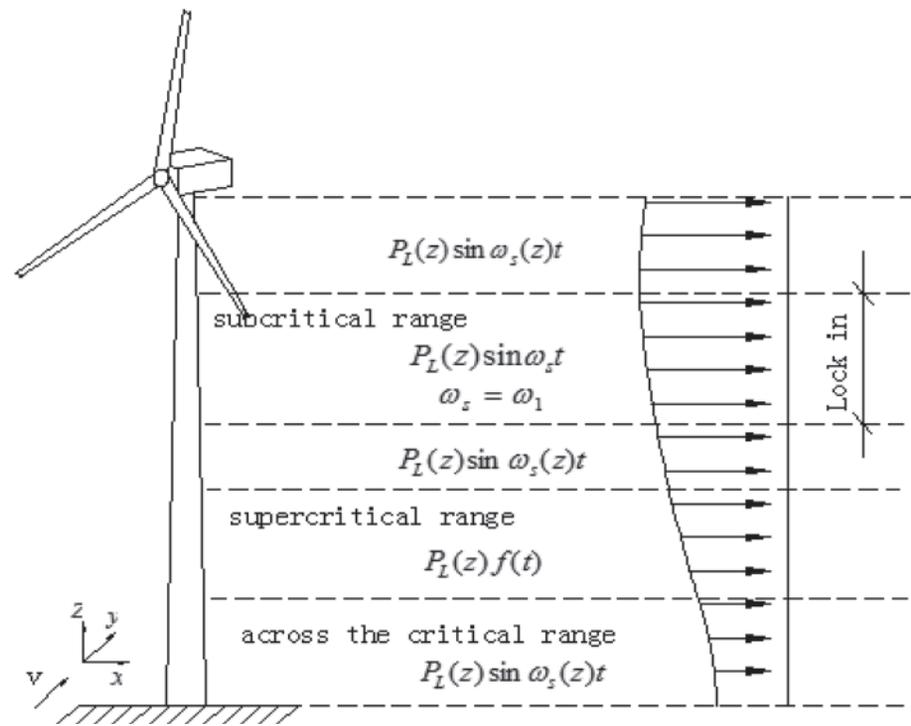
Fig.4: Schematic diagram of transverse wind partition
