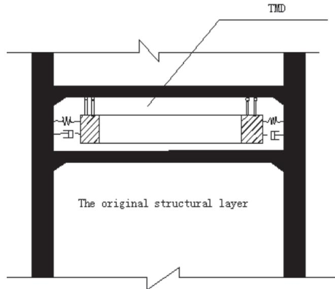
Fig.5: Pendant frequency modulation mass damper of tower tube of wind generator
