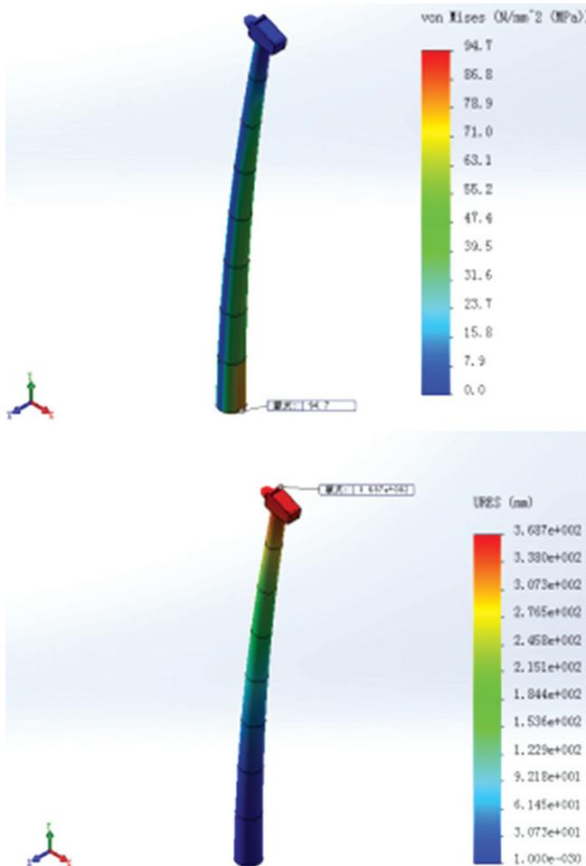
Fig.7 Stress and displacement of tower structure under the rated condition
