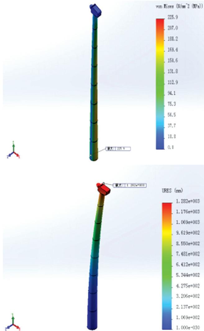
Fig.8: Stress and displacement of the tower structure without damper under the limit condition
