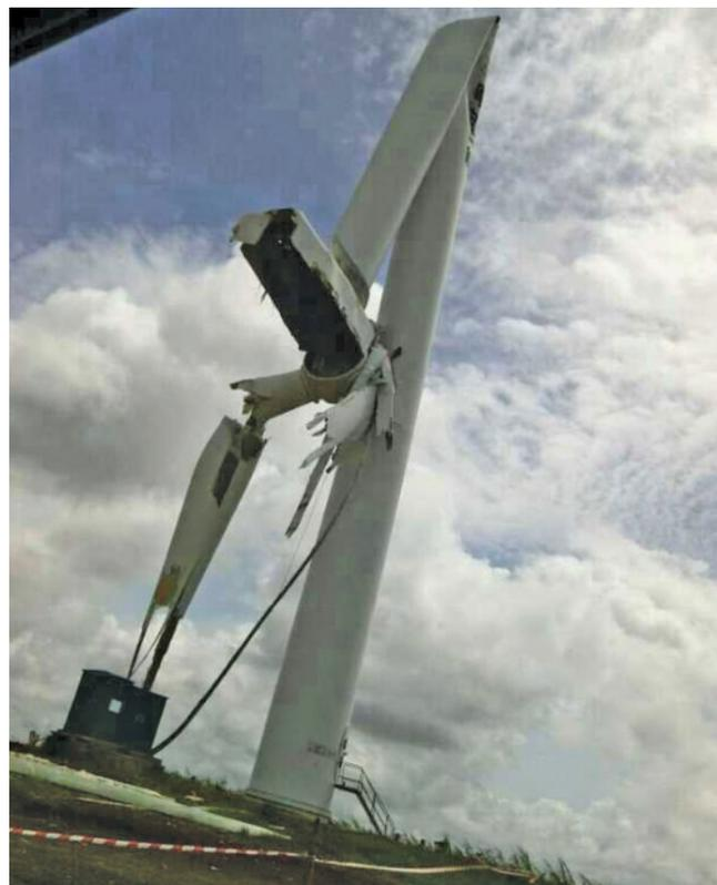
Fig.1: Collapsed tower tube of wind generator caused by typhoon 'catfish'
