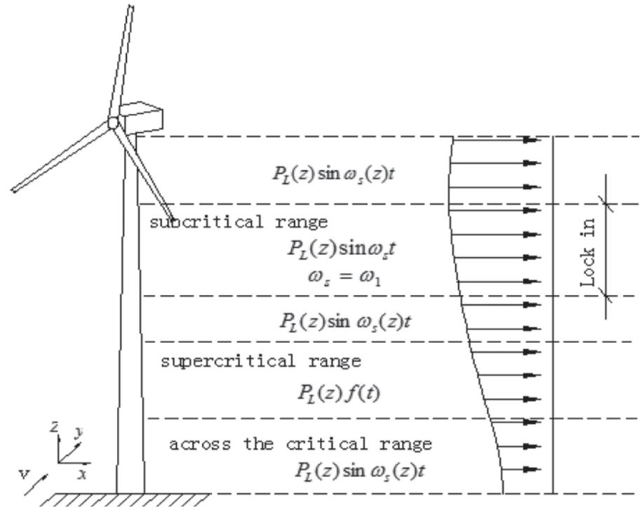
Fig.4: Schematic diagram of transverse wind partition
