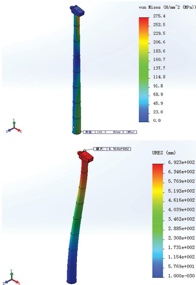
Fig.9: Stress and displacement of the tower structure with damper under the limit condition
