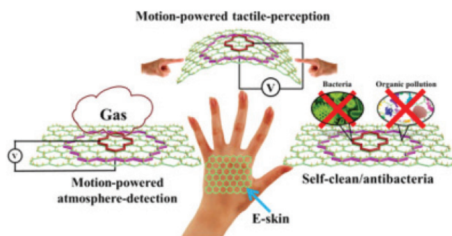
Figure courtesy: Nano Energy, Volume 31, January 2017, Pg.37-48, authors: HaoxuanHe et al A flexible self-powered T-ZnO/PVDF/fabric electronic-skin with multi-functions of tactile-perception, atmosphere-detection and self-clean
