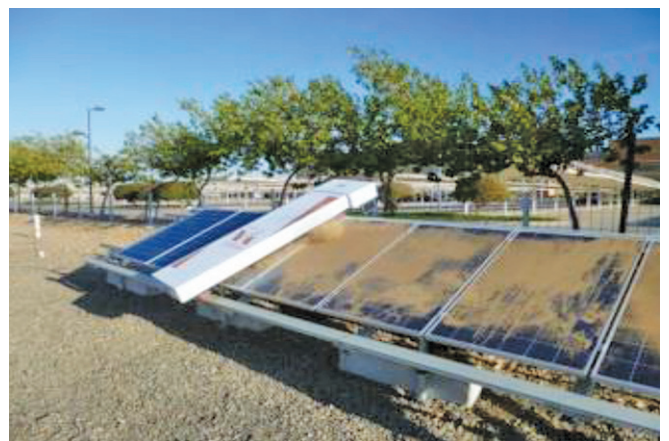
Fig.2: No water automated mechanical dusting device
