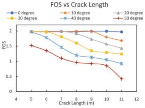
Fig.7 Graphis showing the relation between crack length and crack inclination with FOS
