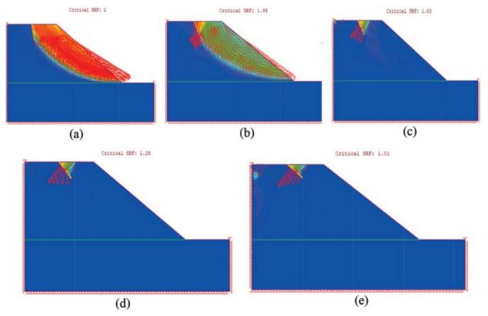
Fig.6 Simulation results with FOS and deformation vector at 15m crack location for crack inclination 10°, 20°, 30°, 40° and 50° in the figure (a), (b), (c), (d) and (e) respectively
