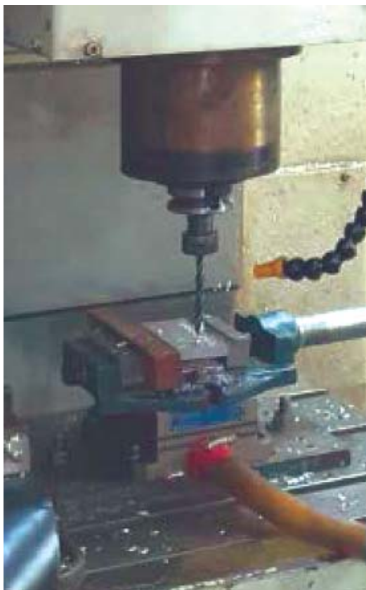
Fig.1 Experimental set up showing the drilling of Al alloy
