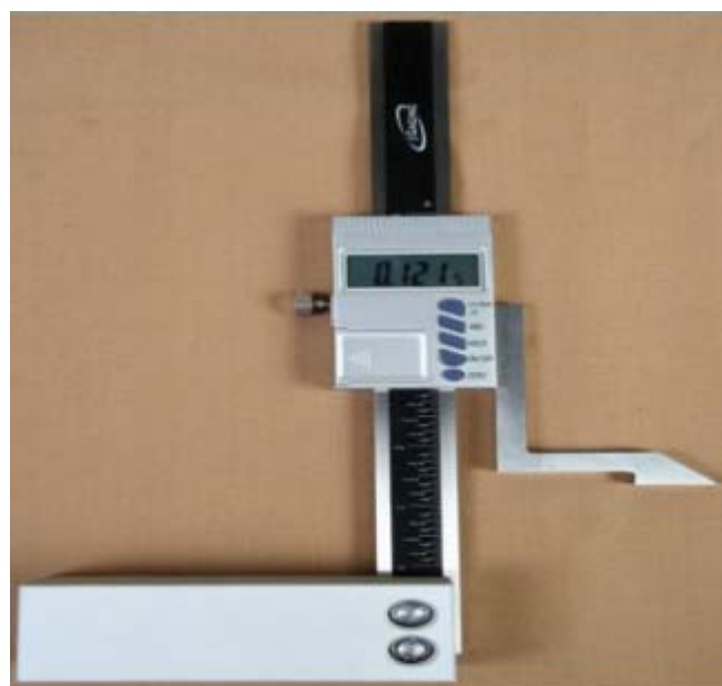
Fig.2 Measurement of burr height using height gauge
