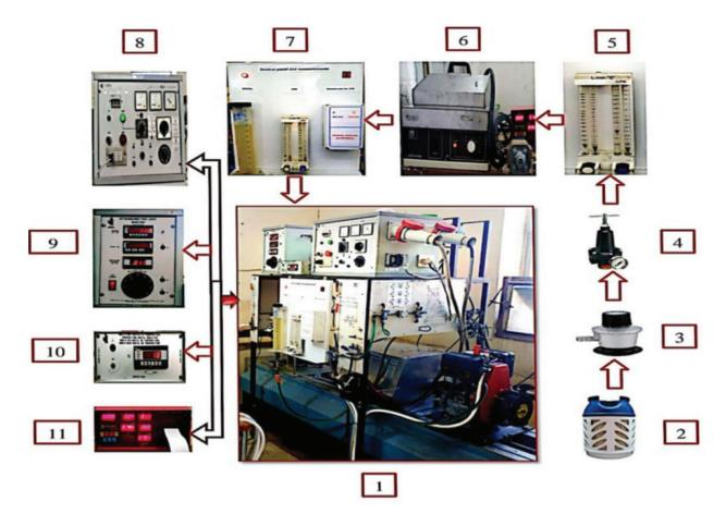
Laboratory device T85D; 2. LPG cylinder; 3. Regulator 4. Pressure regulator and gage; 5. Flow meter for LPG; 6. Vaporizer; 7. Electronic control unit for LPG; 8. Control board; 9. Control of torque; 10. Indicate temperature; 11. Gas analysis.
