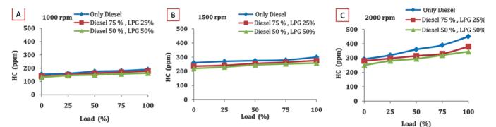
Fig.7 HC emission variation depending on engine load
