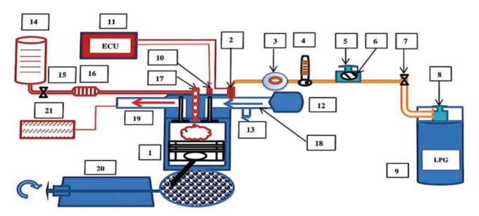
Test engine, 2. LPG injector, 3. Vaporizer, 4. Flow meter for LPG. 5. Pressure regulator, 6. Pressure gage, 7.Valve for LPG, 8. Pressure valve, 9. LPG cylinder, 10. Magnetic senso, 11. Electronic control unit for LPG, 12. Air filter, 13. Air manometer, 14. Diesel flow meter, 15. Diesel valve, 16. Diesel filter, 17. Diesel injector, 18. Intake, 19. Exhaust, 20. Dynamometric unit, 21. Gas analysis unit
