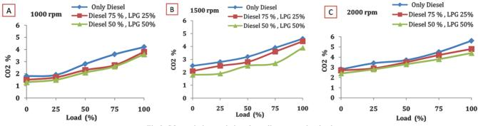
Fig.9 CO<sub>2</sub> emission variation depending on engine load
