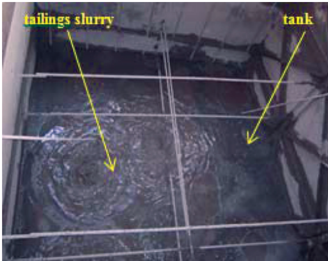
Fig.5 Slurry making through an air compressor
