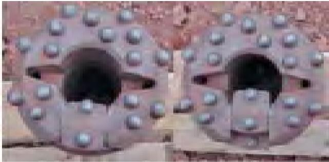
Fig.15 Sliding-block reverse-circulation drilling bit
