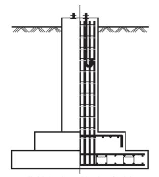
Fig.3 Independent straight column foundation
