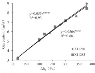
Fig.5 Fitting curves between  $\Delta h_2$  and gas content of different coal samples
