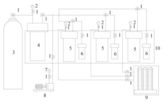
Fig.2 Schematic diagram of gas adsorption and desorption experiment. (1) High-pressure cut-off valve; (2) Accurate pressure meter; (3) High-pressure methane bottle; (4) Gas tank; (5) Big coal sample tank; (6) Small coal sample tank; (7) Vacuum meter; (8) Vacuum pump; (9) Desorption instrument; (10) Thermostatic bath
