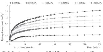
Fig.3 Gas desorption curves of X11283 coal sample under different equilibrium pressure
