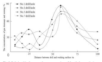
Fig.5 Relationship between the concentration of borehole gas drainage and the distance between the drill field and the working face
