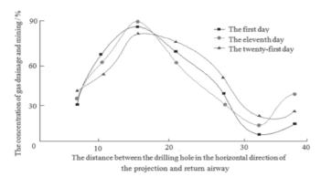
Fig.6 Relationship between the gas extraction concentration and the distance between the final hole drilling and the air return roadway in September
