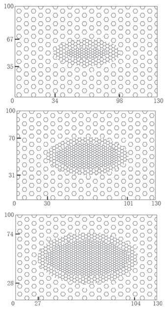
Fig.3 Spatial distribution pattern of the mining-induced fractures "O" form circle diagram with drawing speeds of 2, 4, 6 m/d
