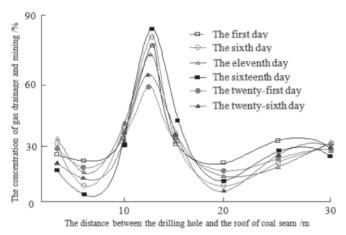
Fig.7 Relationship between the gas extraction concentration and the distance between the final hole drilling and the coal seam roof in no.5 drilling field in September
