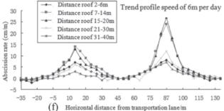
Fig.4 Curves of overlying strata separation rate at the pane advancing 120 m with drawing speeds of 2, 4, 6 m/d
